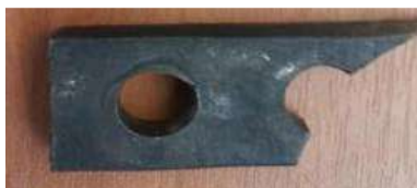
Graphic 6. Stress concentrators in blades.
